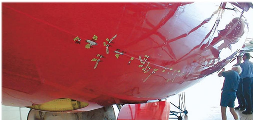
Damage caused by Lightning moving along an airplane
